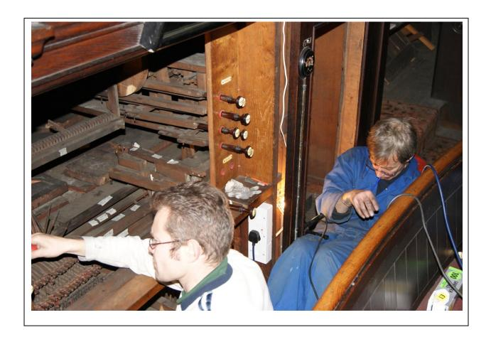
Organ builders (or in this case dismantlers) from David Wood of Huddersfield began work dismantling the organ on 18 October. The patient task of labelling, photographing and removing has taken two weeks. The parts are to be taken to Wood's workshop and repaired, or replaced, before the organ is reassembled next year – possibly as early as March. How we look forward to its renewal!
